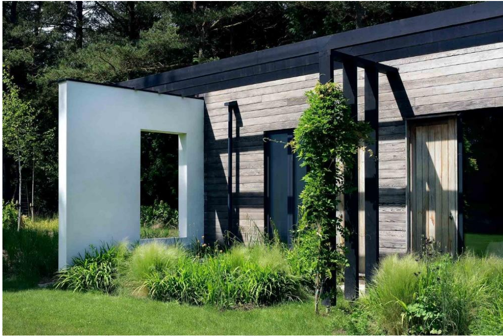
A design with windows oriented to make the most of solar gain, but which are shaded with a pergola to avoid overheating the internal space
