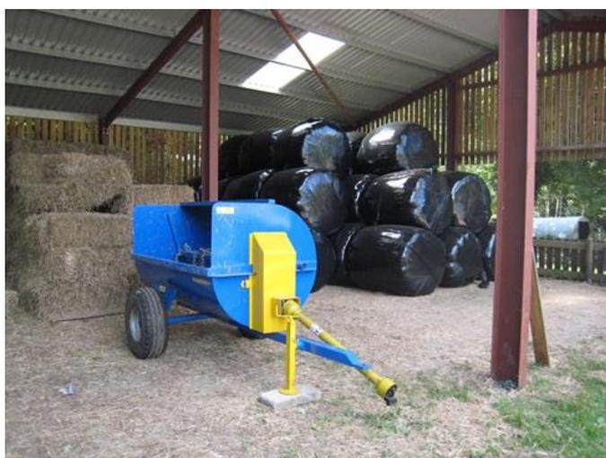
*Modified slurry spreader to distribute pig waste in a way to limit run off and leaching that might effect water quality and wetland plants.*
