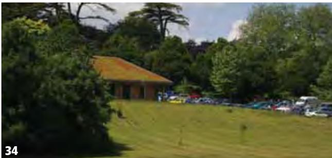
A green roof can help a building merge with landscape. It can encourage rain water filtering and recycling via shallow or steeper pitched solutions. It can also provide effective insulation and sound deadening qualities.
